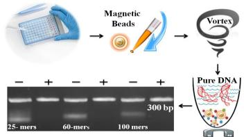
Fig.1 One-Step PCR Cleanup Kit
